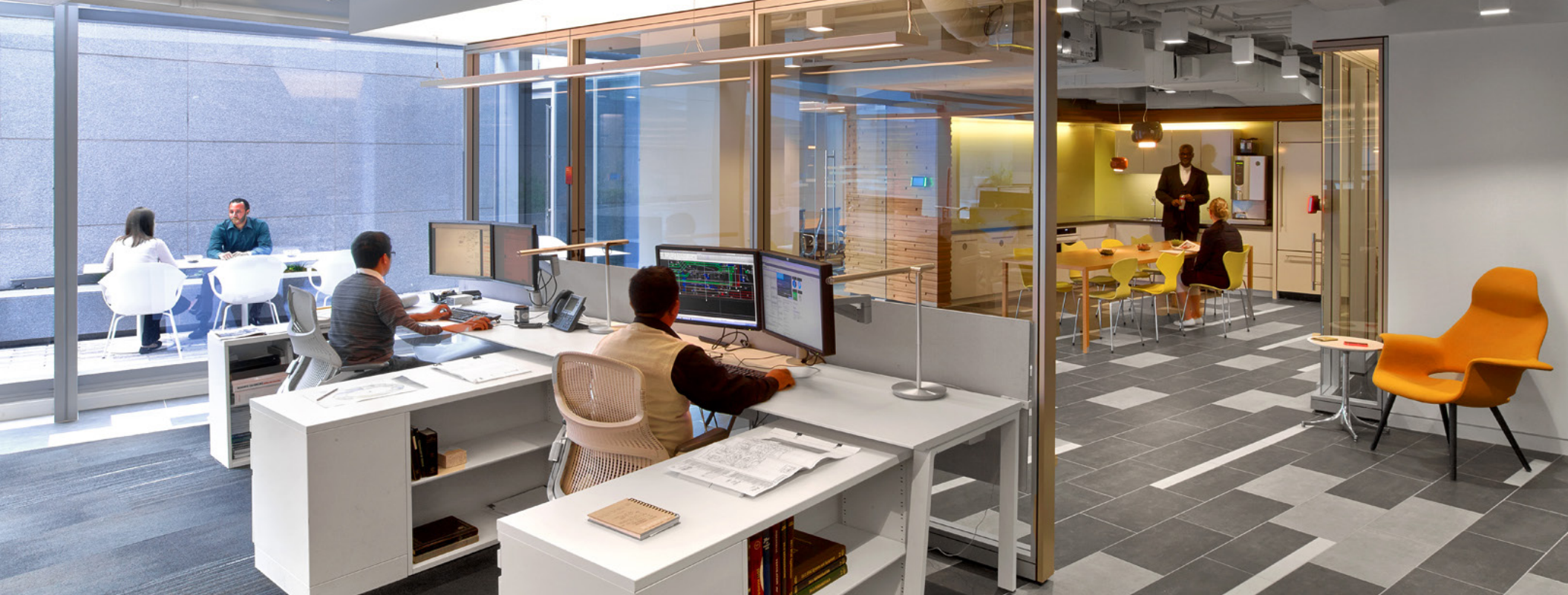
Open Plan | Workstations are perpendicular to windows and all meeting spaces have at least one glass wall to allow daylighting deep into the plan.
