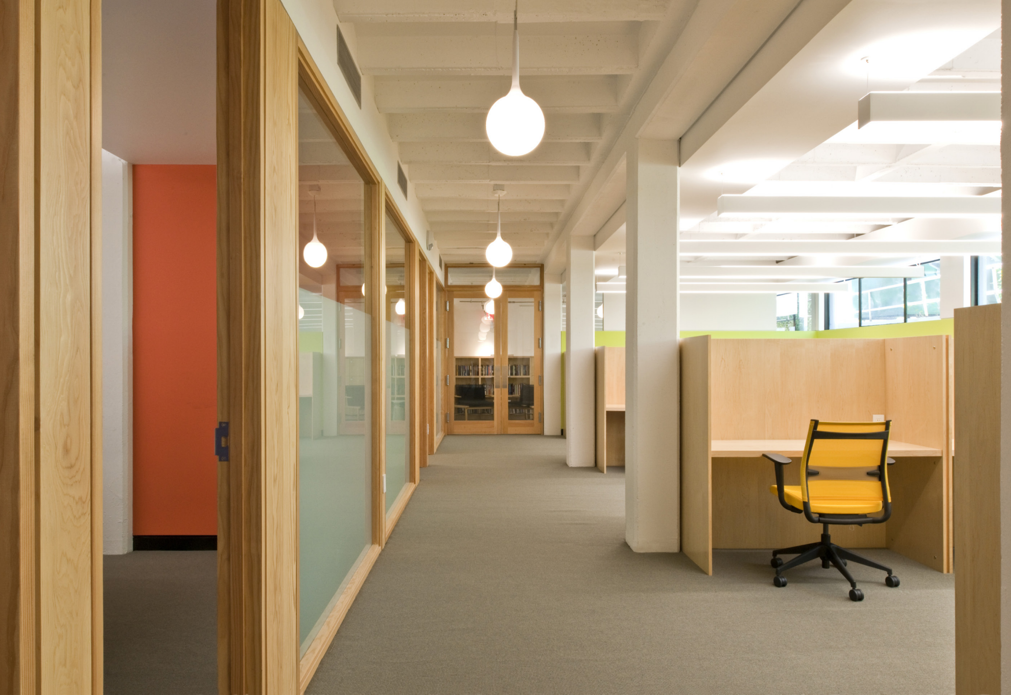
The lower level, renovated as the first phase, now houses a Writer's Studio and new classrooms and offices. Glass walls in Douglas fir frames maximize the available natural light.
